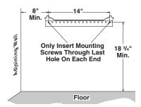
20,000 Btu/hr Models Figure 8 - Mounting Bracket Clearances
